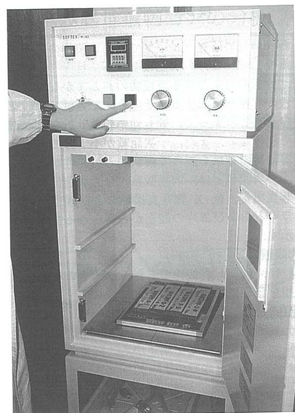
図3 軟 X 線写真撮影の作業風景 Fig.3 Operation of soft x-ray photography device.
